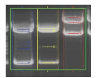
Use the 1D Analysis function to automatically find and label lanes and bands. Easily adjust the parameters.
