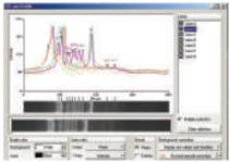
Use the 1D Analysis Lane Profile Graph to generate graphical representation of lanes and bands data.
